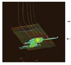
Fracturing begins to develop at the treatment well after pressurizing the depleted area.
