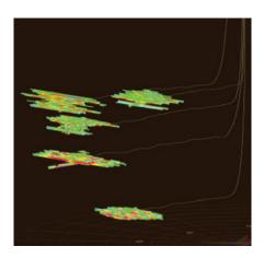
This image shows the ability to model any number of well layers, wells and stages with GOHFER® fracture modeling software.
