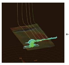
Early pad fluid hits offset depleted well, prior to significant geometry being developed at the treatment well.
