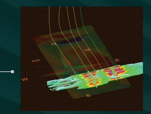
Interference (zipper frac) between wells 1 and 4 causes fracture asymmetry.
