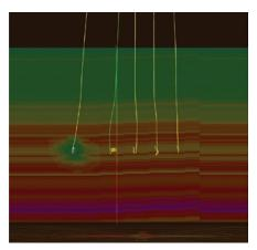
This illustration depicts the offset well depletion effect on total stress (note that there is one fault displayed in this section).
